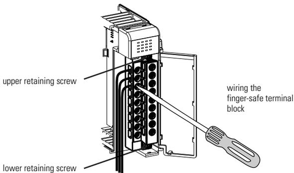
When wiring the terminal block, keep the finger-safe cover in place.
