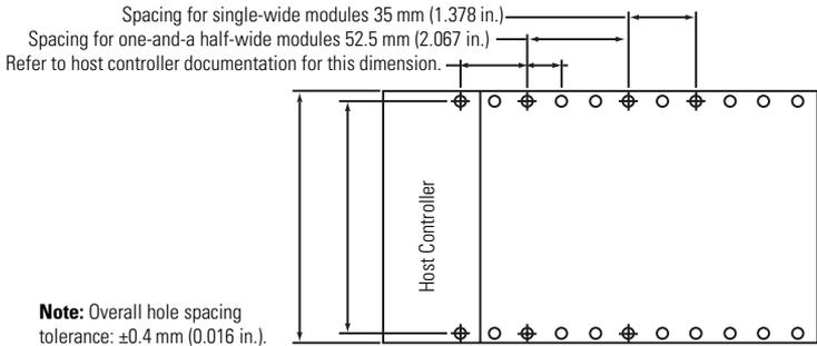
Locate holes every 17.5 mm (0.689 in.) to allow for a mix of single-wide (e.g. 1769-IQ16) and one-and-a-half-wide modules (e.g. 1769-OA16).
