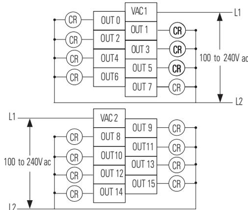
(1) **Surge Suppression** - Connecting surge suppressors across your external load will extend the life of the triac outputs. For additional details, refer to *Industrial Automation Wiring and Grounding Guidelines*, Allen-Bradley publication 1770-4.1.
