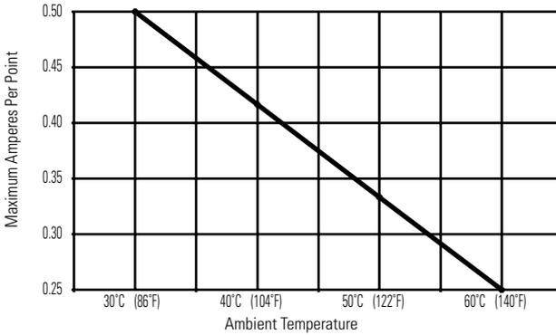
**1769-0A16 Maximum Amperes Per Module vs. Temperature**
