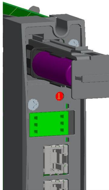
**Note:** Upon power up of a controller which had been powered down with a marginal battery, the initial battery test result will latch and hold for three minutes. This is done so that subsequent battery checks will not falsely indicate “Good”, should the battery voltage recover after removal of the load. After the 3 minute wait period, battery removal and replacement with a new battery will restore the battery diagnostic to Good and reset the battery life accumulator.
