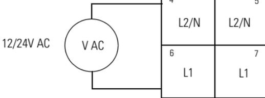
This supply will be connected to the internal field power bus.
