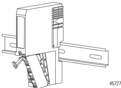
2. Use a small-bladed screwdriver to rotate the DIN rail locking screw to a vertical position. This releases the locking mechanism.
