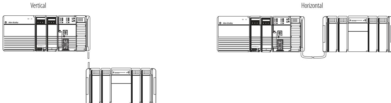
How you orient I/O banks determines the expansion cables that you must connect the I/O banks.
