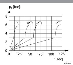
adjustable filling 1) Fully opened p2 = secondary pressure
