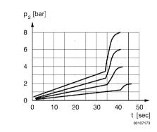
Filling with fixed diaphragm p2 = secondary pressure t = fill time
