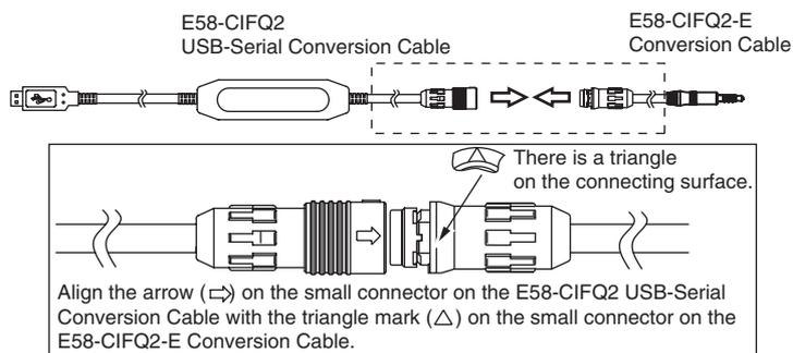
**2** Remove the Port Cover from the front-panel Setup Tool port, and then plug in the Conversion Cable.
