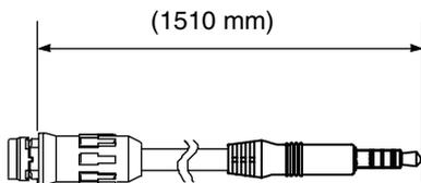
**Connected to the E58-CIFQ2 USB-Serial Conversion Cable**
