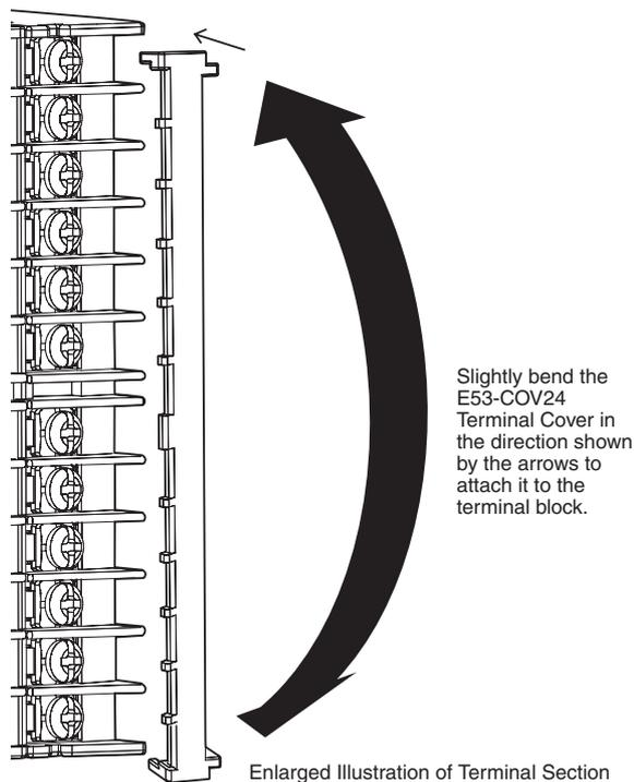
Slightly bend the E53-COV24 Terminal Cover in the direction shown by the arrows to attach it to the terminal block.
