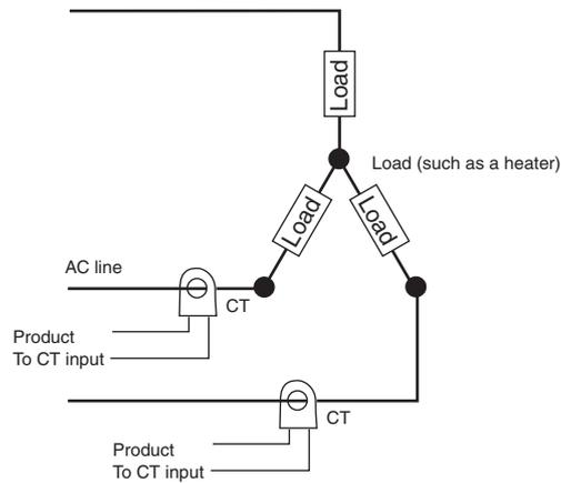
**(c) V connecting lines: Refer to the following diagram for CT installation positions.**
