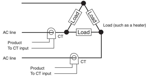
**(b) Star connecting lines: Refer to the following diagram for CT installation positions.**
