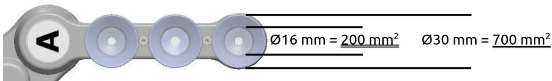
With a typical vacuum of 60% and one vacuum cup with a 200 mm<sup>2</sup> suction area, the lifting force is:
