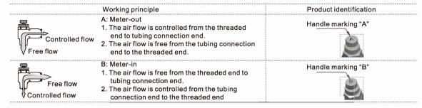
2. Select the different control method according to the actual requirement. The meter-out type is the first priority.
