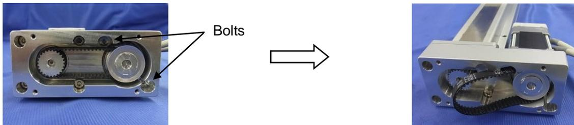
4. After "Belt" is installed, and the bearing support is obtained, the root of "Motor" is pulled in a string or a long banding band. With tensile force adjusted, tighten the bolts which fix the actuator to the motor. (See the table below)
