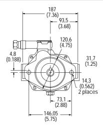
**Note:** Ports are reversed for L.H. rotation. Control location same for both L.H. and R.H. rotation.
