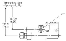
Load sensing comp. control port location for R.H. rotation .4375-20 UNF-2B boss connection
